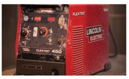
Among other tests, the Flextec<sup>™</sup> 450 was subjected to extreme temperature environmental testing, including heat, cold, humidity, rain and dust.
