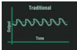
Traditional weld control is more variable around the desired output.
